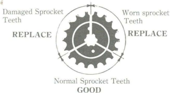
5. If the drive chain or sprockets are excessively worn or damaged, they should be replaced. Never use a new chain with worn sprockets, rapid chain wear will result.
